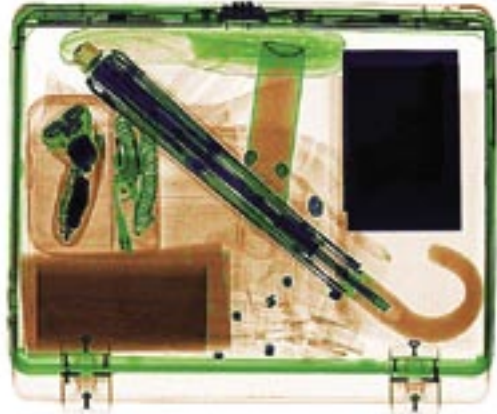
Color image where materials are represented as: orange for organic, blue for inorganic, green for amorphous objects.
