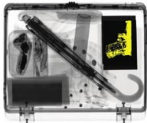
Example of automatic signaling of metallic high-absorption object (adjustable threshold)
